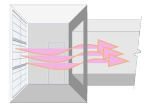
**Upgraded System with (24) high power UVC lamps installed downstream from the Coil** (This cleans the COIL for energy savings and cleans the AIR by maximizing pathogen irradiation in the DUCTS.)
