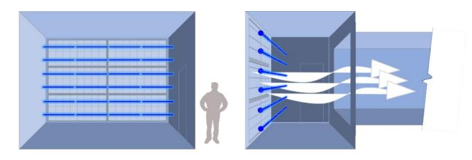
This example above is for a property with multiple air handling units. This particular AHU-1 has three rows of two coils that are each 8' wide  $\times 3.5'$  tall. The six coils are stacked three high in the plenum that is 16' wide  $\times 11.5'$  tall. The CFM is 73,600 and the approximate square footage of the conditioned area for this ACH-1 is 60,000 SF.
