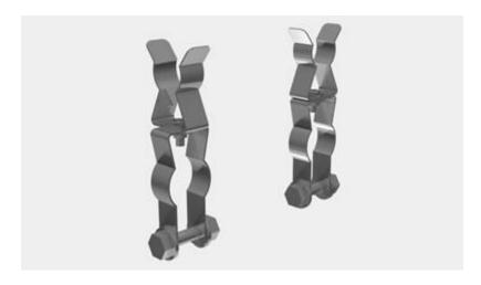
Snap-in stainless steel clips on one side allow tool-free lamp installation and replacement while securely holding lamps. The other side of the clip is made to clamp around standard electrical conduit
