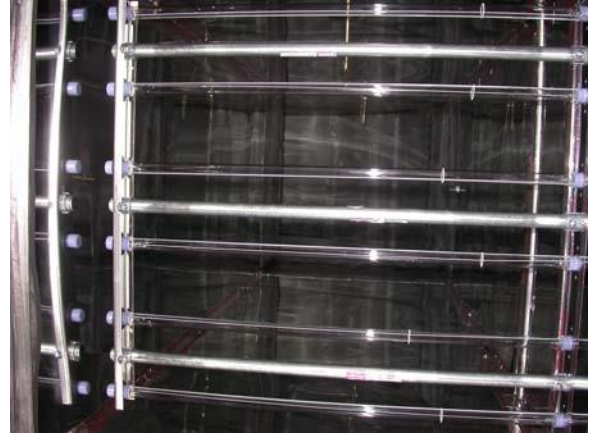
Figure 2-2. Device installed inside the test rig. There are six lamps and three support
