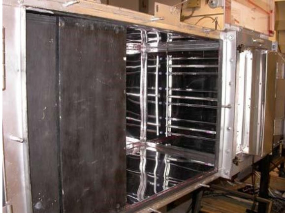
Figure 2-1. Ballast box installed on the outside of the test rig (on right). The rods. is also devise is also visible.
